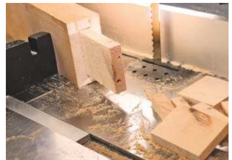
▲ Using the basic mitre fence it's very easy to cut a tenon in a minute or so
